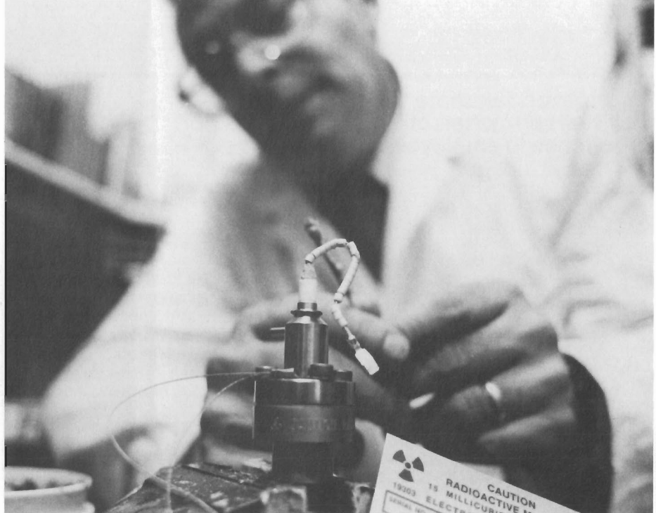
Dave Salonin reassembles a radioactive detector from a gas chromatograph in his new repair center. Low radiation levels inside the steel cylinder detect chemical compounds.
